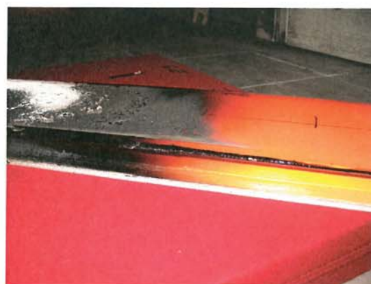
Test material for the cone test (with honeycomb structure) and for spread of flame test (closed structure).
