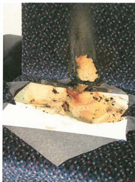
Self-extinguishing after 4:57 minutes
